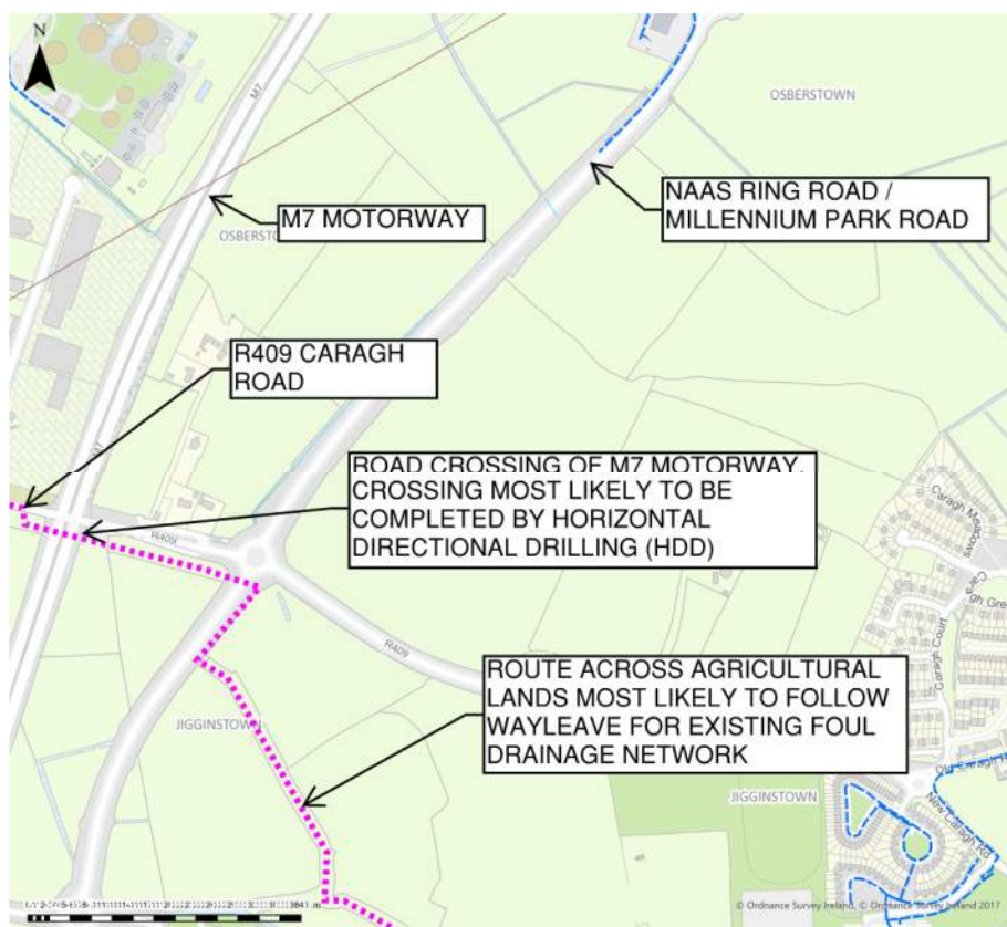
Figure 2-6 - Extract from GNI network map with most likely route for upgraded high-pressure transmission pipeline indicated to Caragh Road
